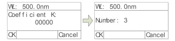
**5)** Calibrate Standard Samples. Put the corresponding standard samples in the light path as the screen indicates, press to input the concentration, press (left) to confirm, to finish all the standard samples.
